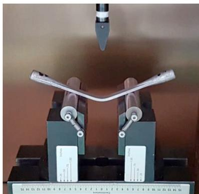
Fig. 3. Dynamic three-point bending test stand with damaged specimen
