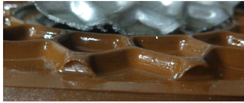
Fig 1 Filleting of the edges after number of deformation cycles
