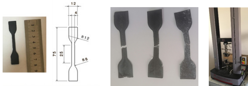
Figure 1. Geometry and the tensile test of a layers ( 45^\circ, 0^\circ, 90^\circ )
